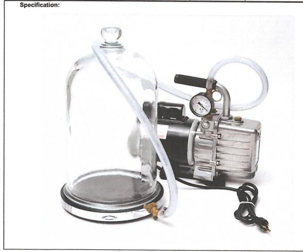
High Vacuum Pump Deluxe Experiment Kit This kit includes everything you need to immediately begin teaching high vacuum physics right out of the box. The kits comes with our LAV-3/G high vacuum pump with a mounted 30" Hg gauge. The pump is a direct drive, two stage rotary van high vacuum pump which can achieve 20 microns in laboratory conditions.
