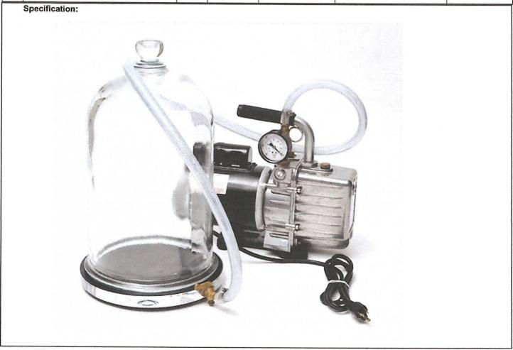
High Vacuum Pump Deluxe Experiment Kit This kit includes everything you need to immediately begin teaching high vacuum physics right out of the box. The kits comes with our LAV-3/G high vacuum pump with a mounted 30" Hg gauge. The pump is a direct drive, two stage rotary van high vacuum pump which can achieve 20 microns in laboratory conditions.
